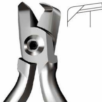
12-6312 T/C 11.5 cm/ 4½" Distal End Cutter with safety hold It shear cuts hard wire and braided wire and then, safely holds the loose distal ends of the wire, thus preventing from falling down into the oral tissues. The cutting edges are diamond honed. Maximum cutting capacity: rectangular and twist wires up to .022 x .028" ( 0.56 x 0.71); round wire up to .020" ( 0.51 mm) in diameter.
