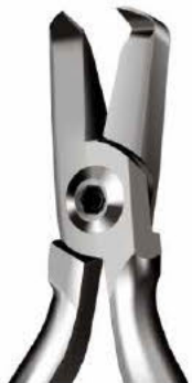
12-6212 T/C 12 cm/ 5" Mini cut & hold distal end cutter cuts with in 0.5mm from end of buccal tube. Use on wire up to 0.22" x 0.28" rectangular and 0.20" round.
